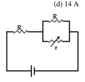
In the circuit shown, the resistance r is a variable resistance. If for r = fR, the heat generation in r is maximum then the value of f is:
