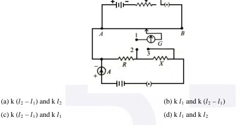
11) In the circuit shown the cells A and B have negligible resistances. For  $V_A = 12V$ ,  $R_1 = 500\Omega$  and  $R = 100\Omega$  the galvanometer (G) shows no deflection. The value of  $V_B$  is:
