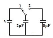
A capacitor of  $2\mu F$  is charged as shown in the diagram. When the switch S is turned to position 2, the percentage of its stored energy dissipated is:
