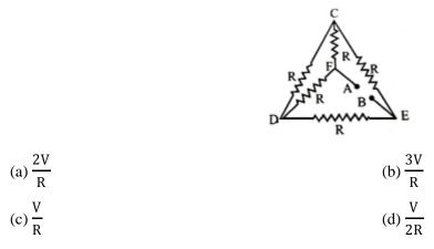
7) For the network shown in the Fig. the value of the current is
