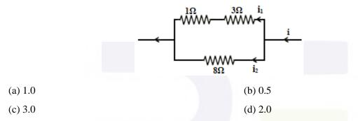
19) The total power dissipated in watts in the circuit shown here is
