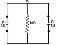
The current in the 10  $\Omega$  resistor is
